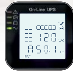
Module Control Panel
